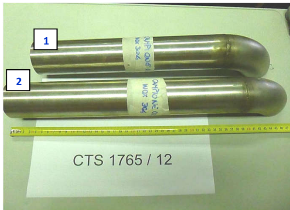
AISI 304L samplings from the onboard installation
