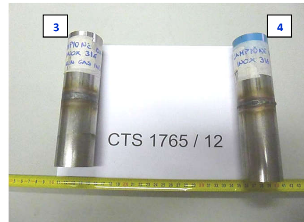
AISI 316L samplings from the proposed repairing
