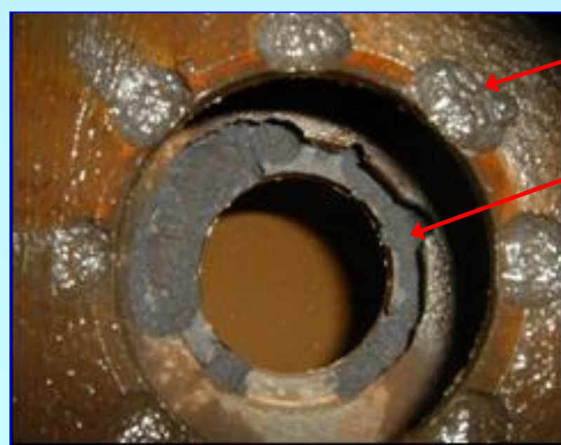
Corrosion morphology in Intermediate phase Broad Corrosion morphology
